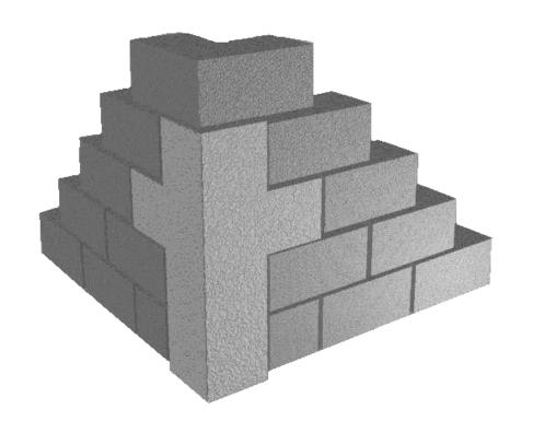
The **cornerstone** (or foundation stone or setting stone) is the first stone set in the construction of a masonry foundation, important since all other stones will be set in reference to this stone, thus determining the position of the entire structure.
